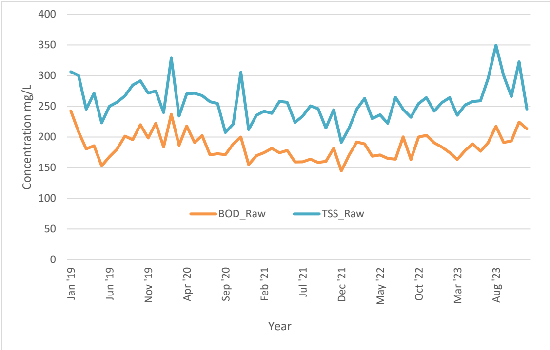
Figure - 3 WwTF Average Monthly Influent Five-Day Biochemical Oxygen Demand and Total Suspended Solids Concentrations (mg/L)
