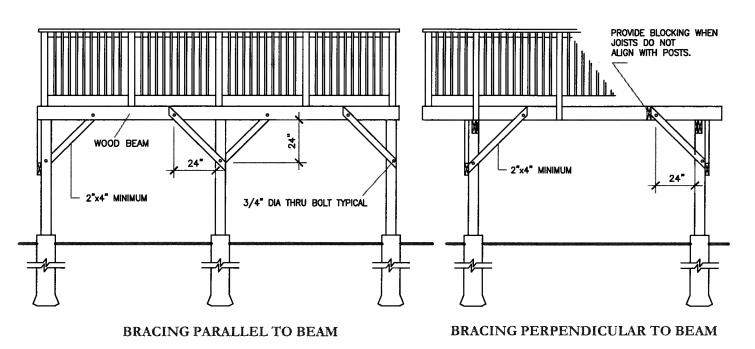
DECKS GREATER THEN 24" ABOVE GRADE SHALL BE PROVIDED WITH LATERAL BRACING TO ENSURE DECK STABILITY
