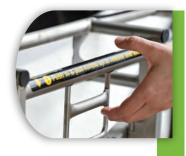
While holding your bike with one hand, squeeze the holding to release the latch lower the rack.
