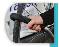
To unload your bike, raise the support arm off the tire and move it down and out of the way.
