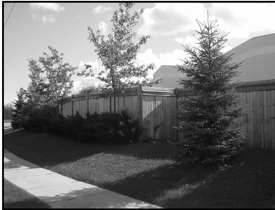
The visual impact of this fence is reduced through changes in plane and landscape massing.
