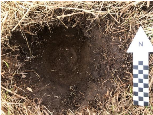
Image 15: Typical test pit – 30 cm of dark brown sandy loam above orange sandy clay subsoil.
