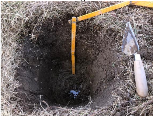
Image 5: Typical test pit – 25 cm of dark brown loam/muck above grey sandy clay subsoil. Water present 10-15 cm into subsoil indicating proximity to low-lying wet areas.
