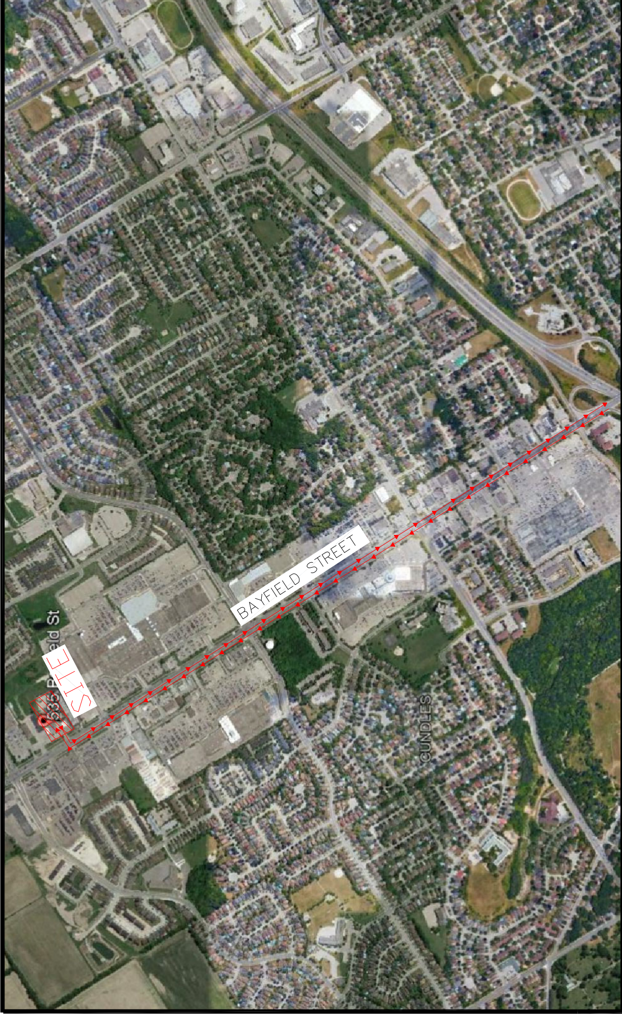
Figure 10 - Proposed Construction Traffic (Truck) Route
