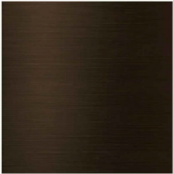
2. DARK BROWN METAL (Window mullions, pre-finished metal panels, canopy finish, slab edge cover)
