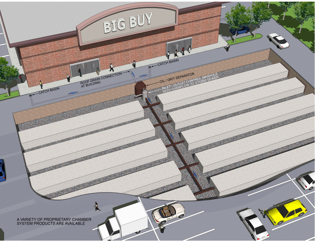
Infiltration Chamber System Under Parking Lot
