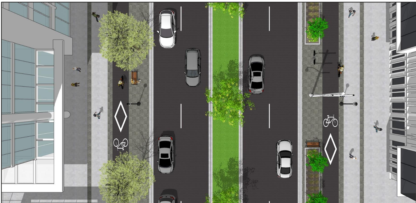
Exhibit 6-9: Bradford Street Typical Cross-section Aerial View
