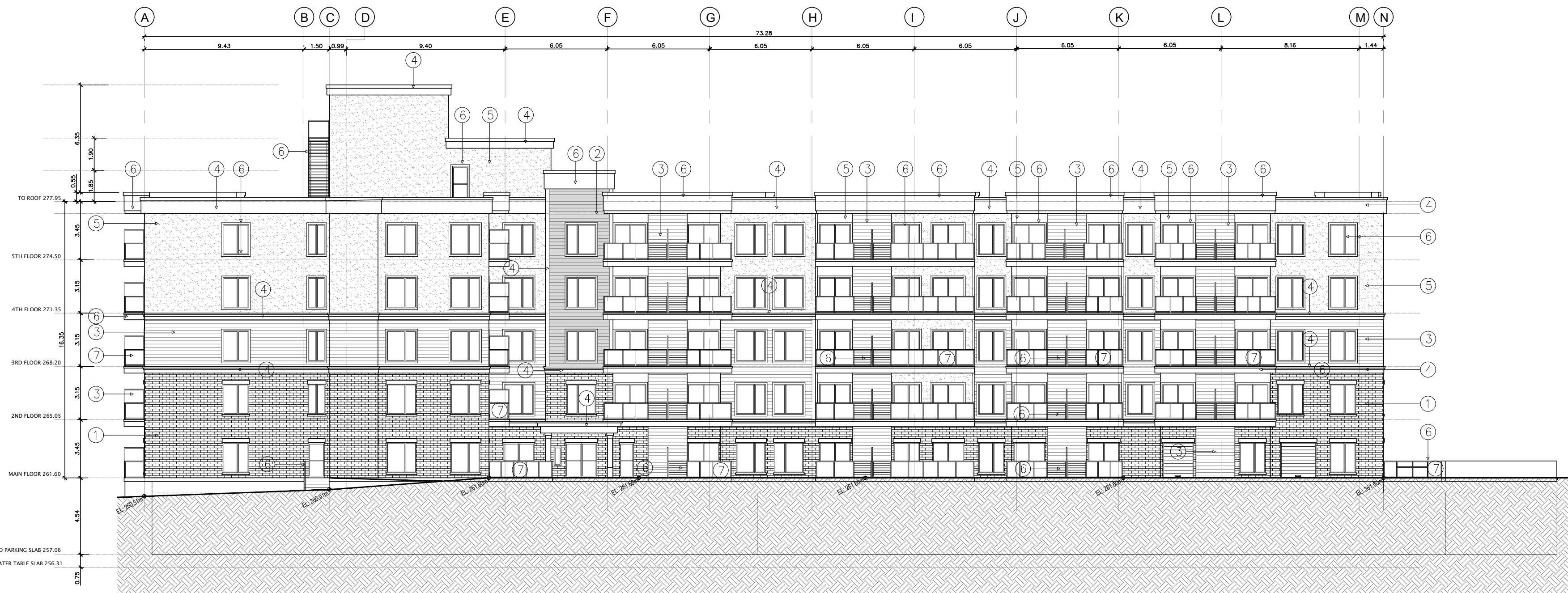
SOUTH ELEVATION FROM COURT YARD
