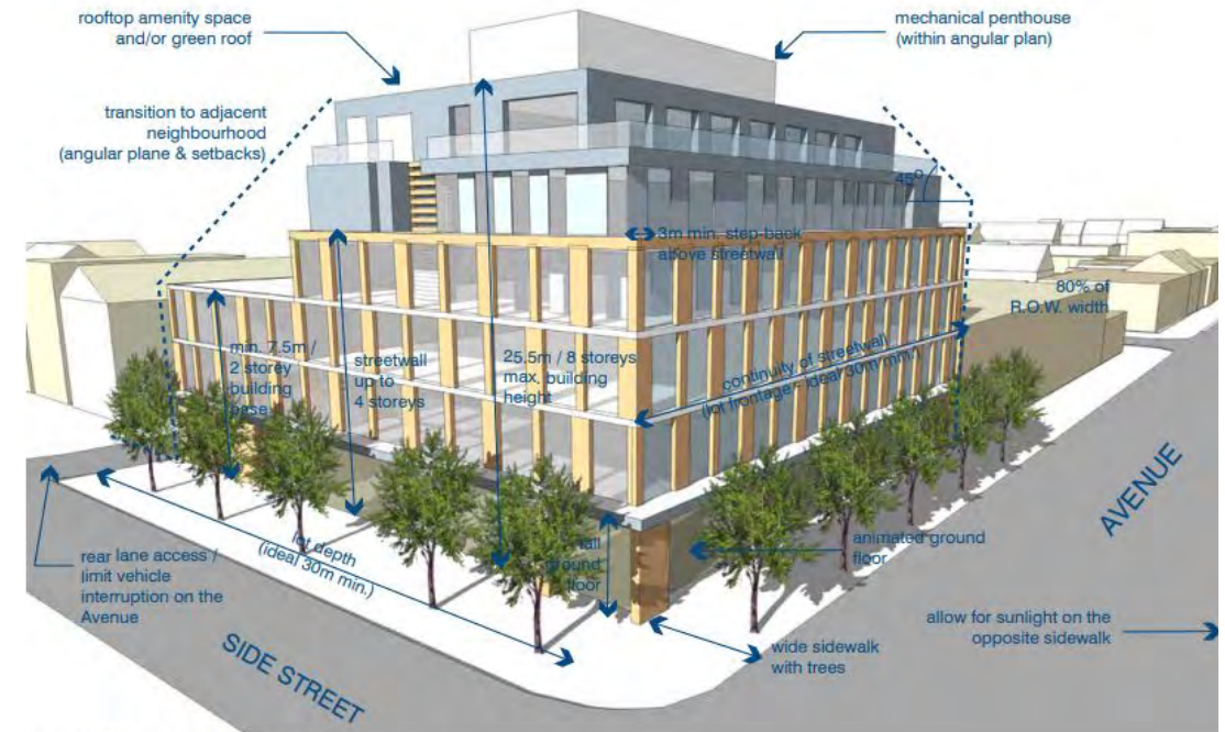
Figure 38: Sample Building Articulation Diagram depicts some of the key components of the guidelines affecting the built form.
