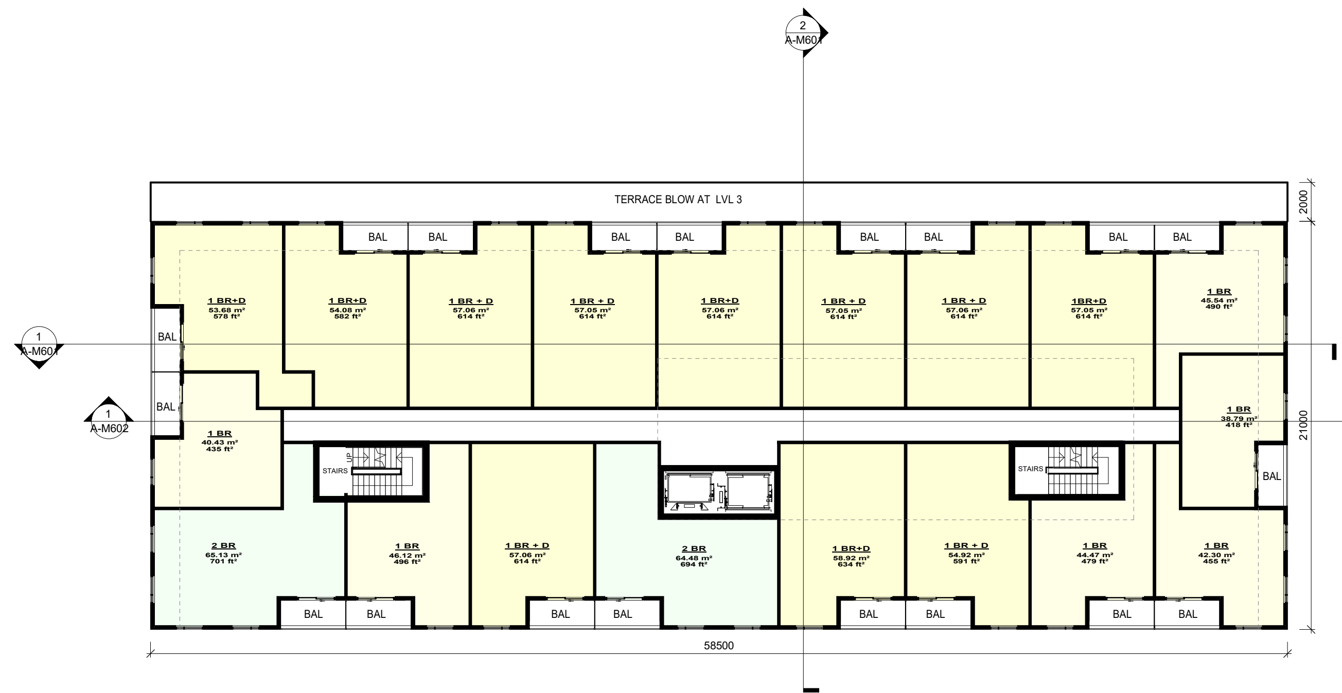
2 TYPICAL LEVEL 4, 5 FLOOR PLAN 1 : 200
