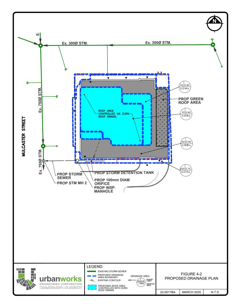
Rooftop **Proposed** Storage Storage # of Storage ID Area Release Rate Required **Provided** notches  $(m^3)$ (m<sup>2</sup>) $(m^3)$ (L/s)13.1 Roof 1 508 2 3.7 63.2 1 Roof 2 138 1.9 3.0 17.2 3 Total 646 5.6 15.8 80.4
