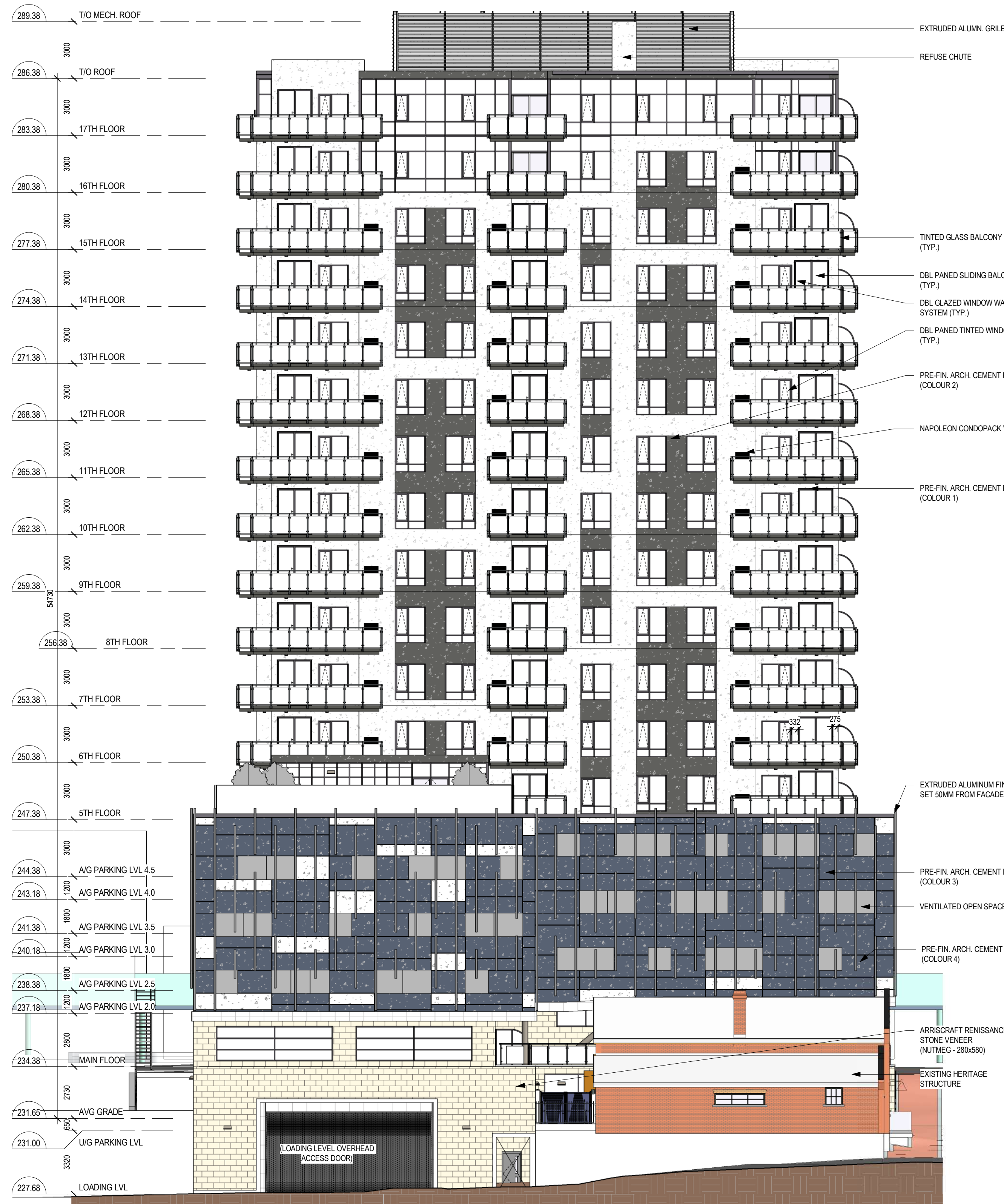
1 SOUTH ELEVATION - COLOURED A3.4 1 : 150
