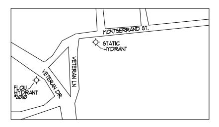
STATIC PRESSURE: 50 PSI UNDERGROUND TYPE & SIZE: 150 mm CPVC
