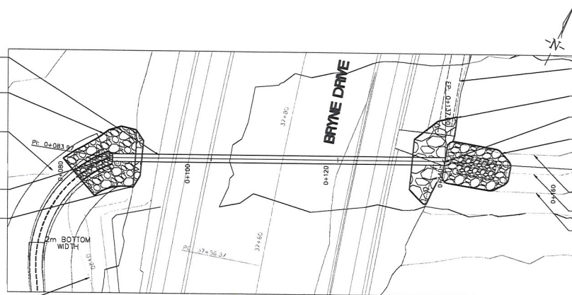
PLAN: LOVERS CREEK CULVERT SCALE 1:250
