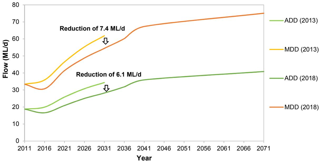
**Figure 3-2 Comparison of 2013 and 2018 Master Plan Surface Water Projections (Southern Zones: 2S and 3S)**
