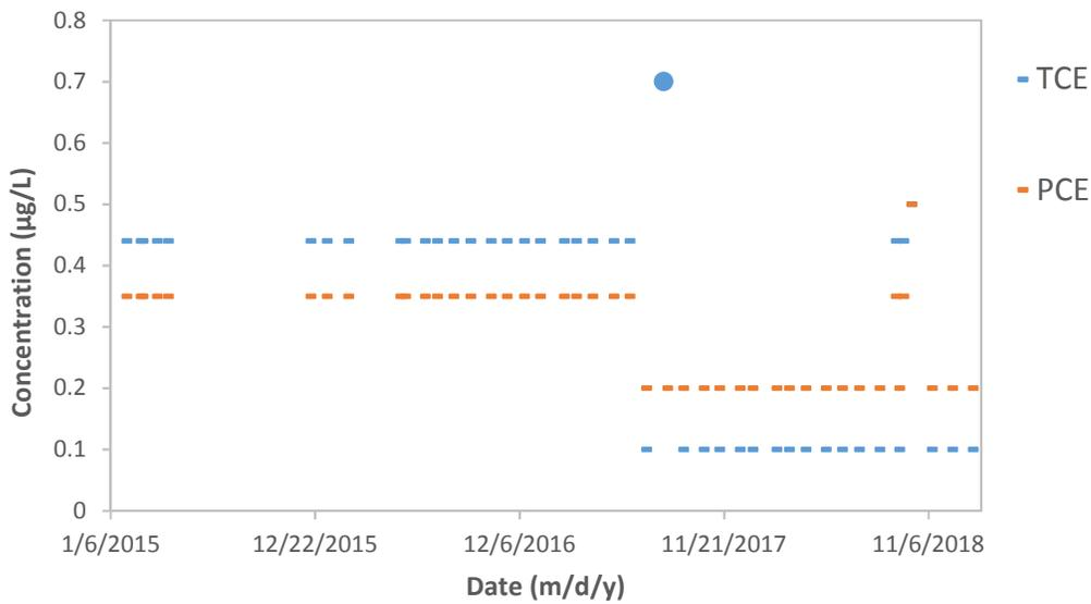
**Figure 2-6 TCE and PCE Concentrations in Well 12 Raw Water from January 2015 to January 2018 (dashed lines represent MDLs; dots represent reported concentrations)**
