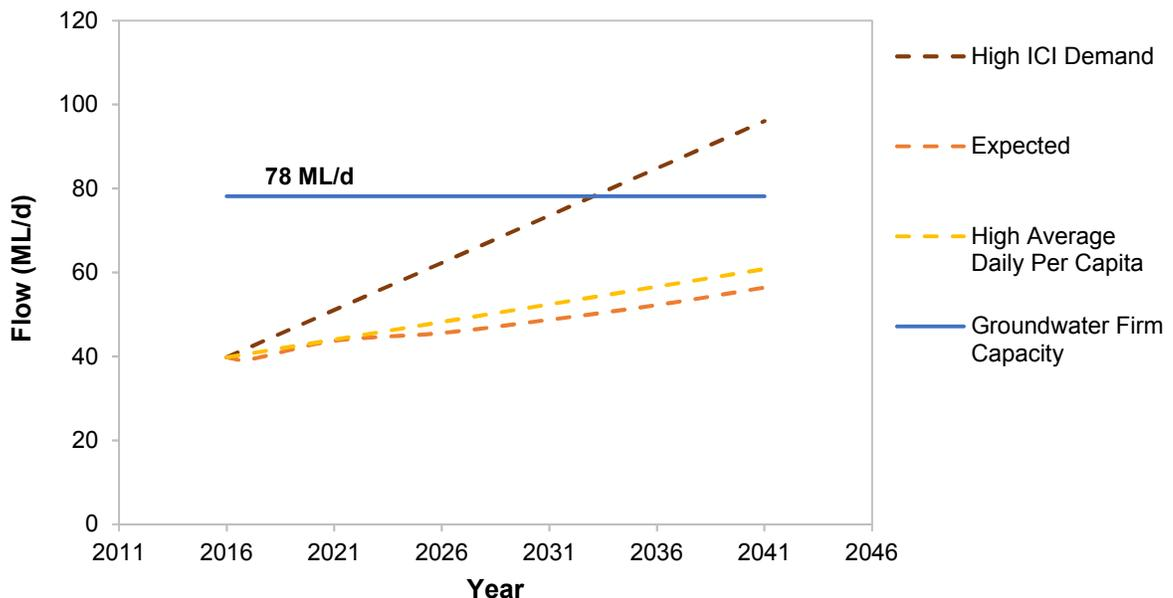
**Figure 4-4 Sensitivity Analysis Displaying Scenarios for the 2041 Northern Zones MDD Flow Projection**
