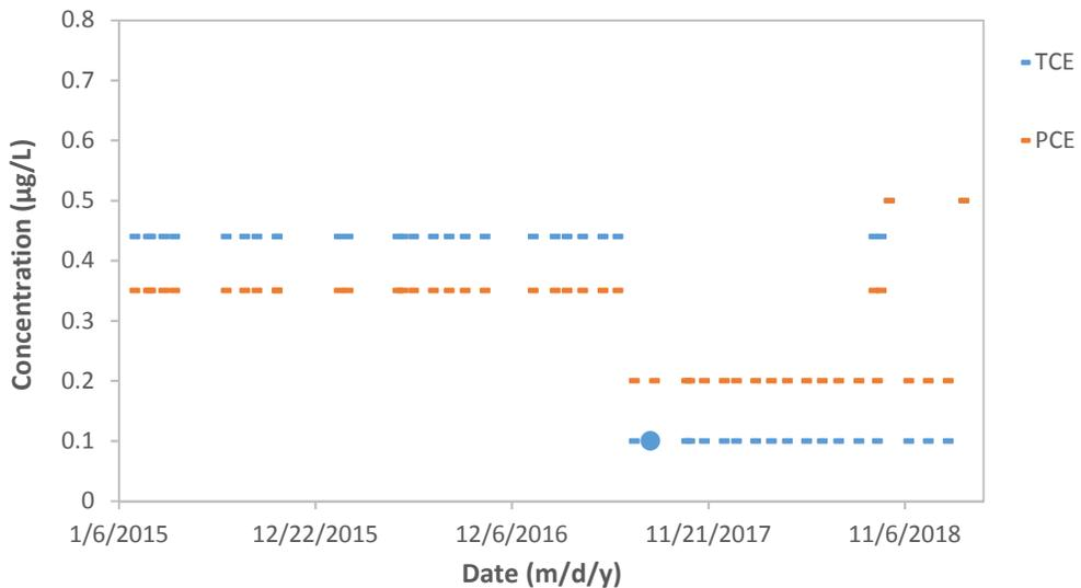
**Figure 2-8 TCE and PCE Concentrations in Well 15 Raw Water from January 2015 to January 2018 (dashed lines represent MDLs; dots represent reported concentrations)**
