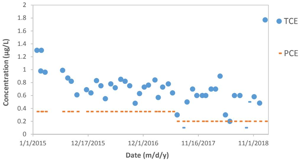
**Figure 2-7 TCE and PCE Concentrations in Well 14 Raw Water from January 2015 to January 2018 (dashed lines represent MDLs; dots represent reported concentrations)**
