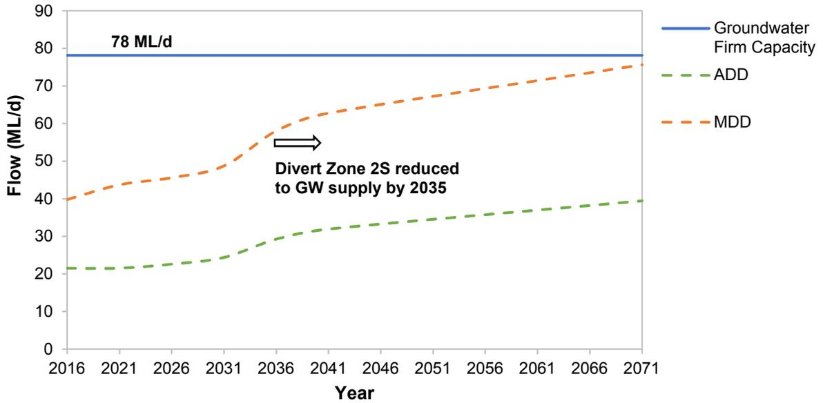
**Figure 5-3 City of Barrie 2018 Groundwater Demand Projections compared to Groundwater Firm Production Capacity (Northern Zones: 1, 2N, and 3N) with the implementation of Alternative 5**
