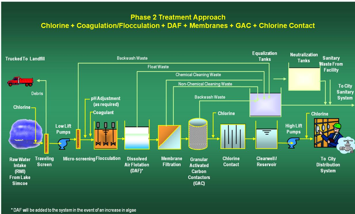
Figure 2-3 Process Schematic of Surface Water Treatment Plant
