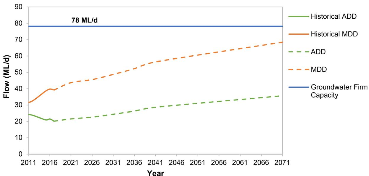
Figure 4-1 City of Barrie 2018 Groundwater Demand Projections (Northern Zones: 1, 2N, and 3N) compared to Groundwater Firm Production Capacity
