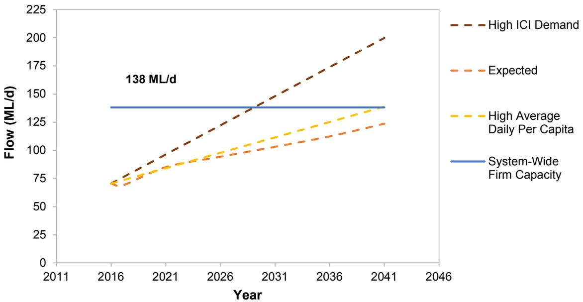
**Figure 4-6 Sensitivity Analysis Displaying Scenarios for the 2041 System-Wide MDD Flow Projection**
