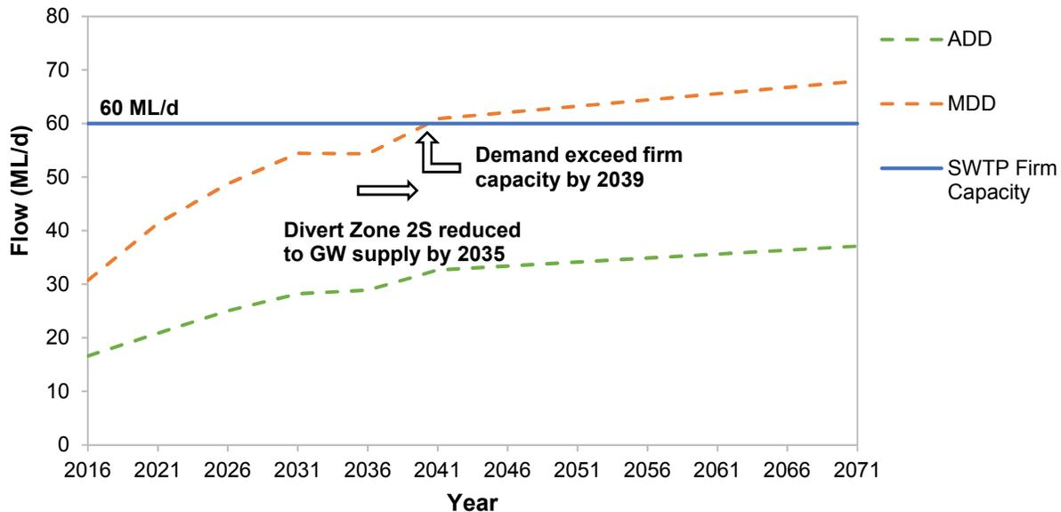
**Figure 5-4 City of Barrie 2018 Surface Water Demand Projections compared to SWTP Firm Production Capacity (Southern Zones: 2S, and 3S) with the implementation of Alternative 5**
