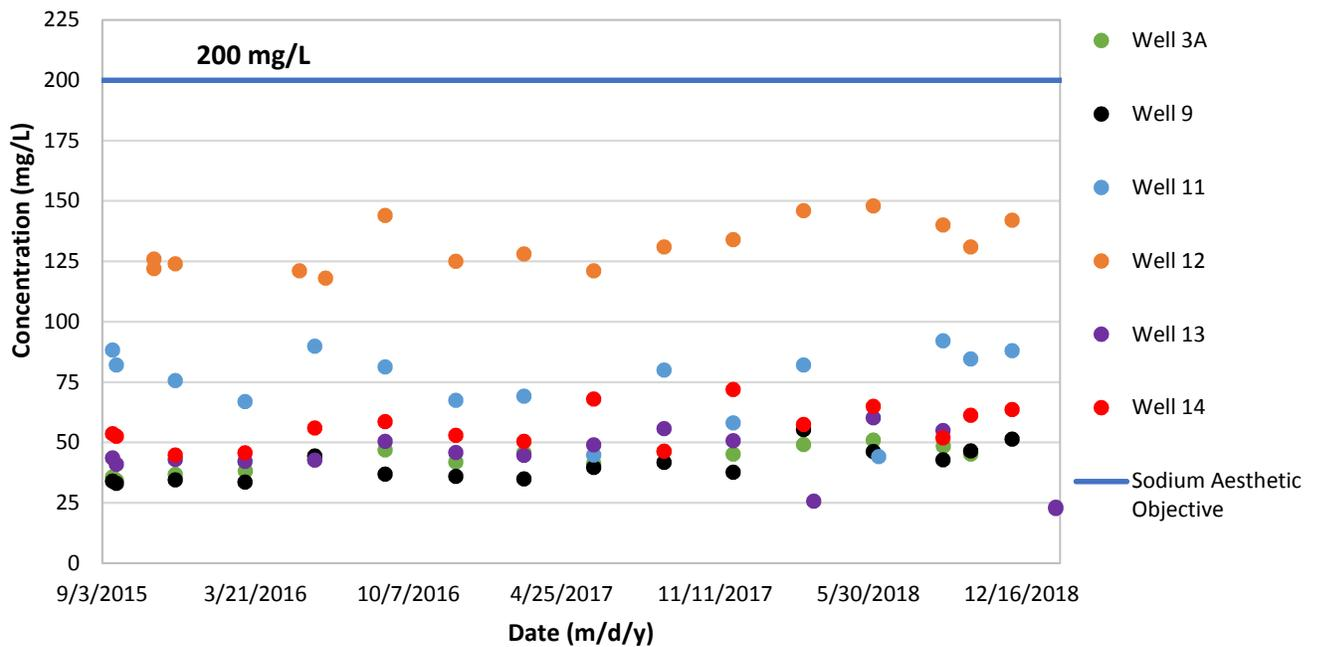
**Figure 2-4 Sodium Concentrations in Raw Water from 2015 to 2018 for Wells 3A, 9, 11, 12, 13, and 14**
