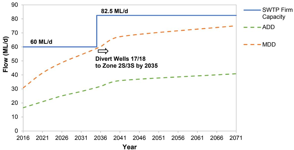
**Figure 5-6 City of Barrie 2018 Surface Water Demand Projections compared to SWTP Firm Production Capacity (Southern Zones: 2S, and 3S) with the implementation of Alternative 6A**
