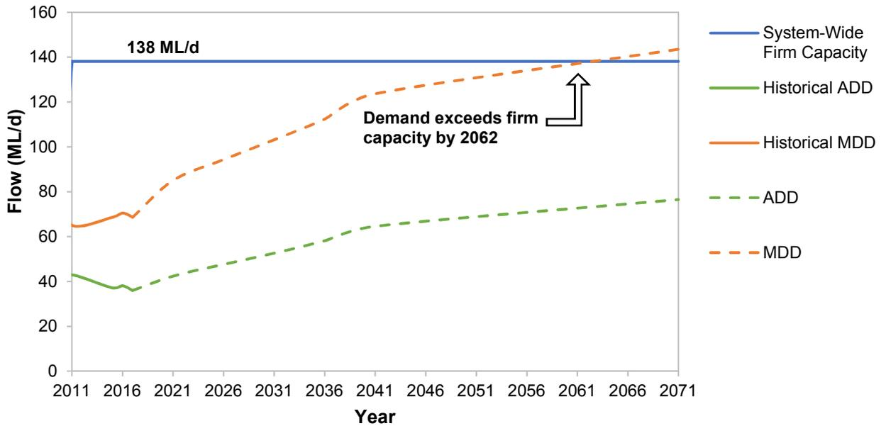
**Figure 4-3 City of Barrie 2018 System-Wide Water Demand Projections compared to System-Wide Firm Production Capacity**
