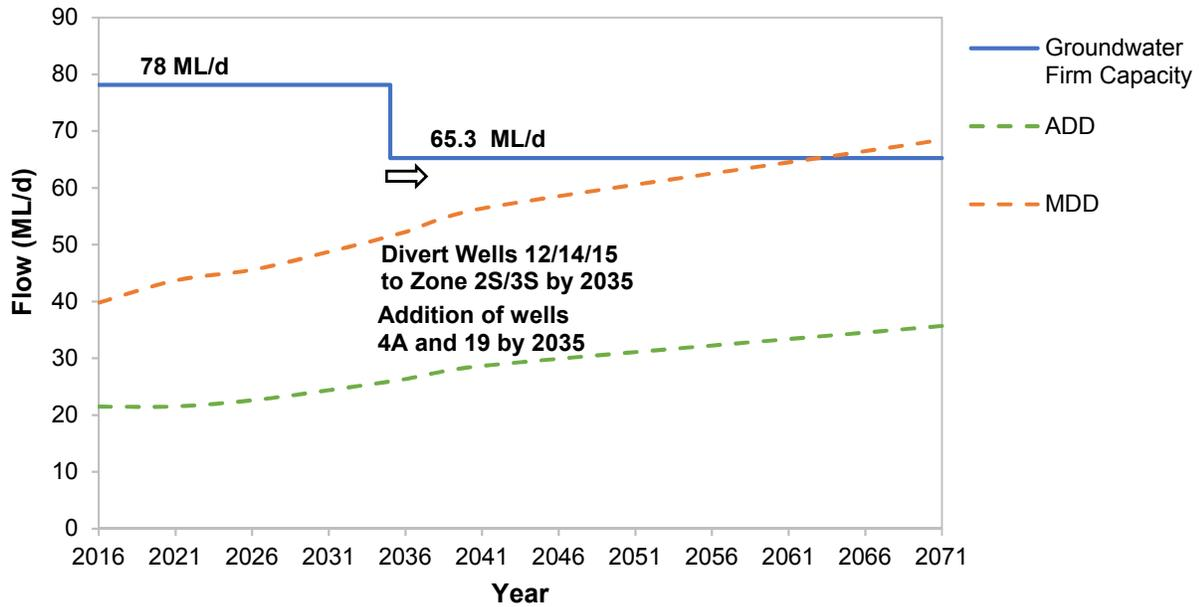
**Figure 5-7 City of Barrie 2018 Groundwater Demand Projections Compared to Groundwater Firm Production Capacity (Northern Zones: 1, 2N, and 3N) with the implementation of Alternative 6B**
