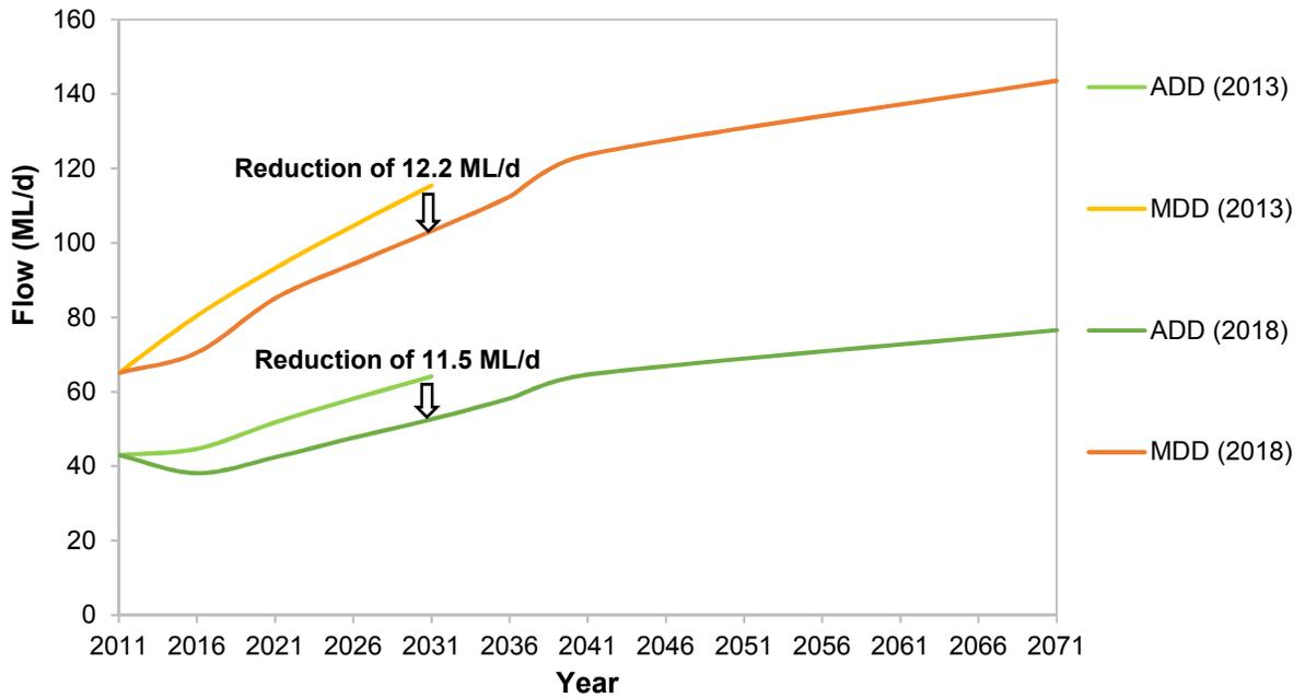
**Figure 3-3 Comparison of 2013 and 2018 Master Plan System-Wide Projections**
