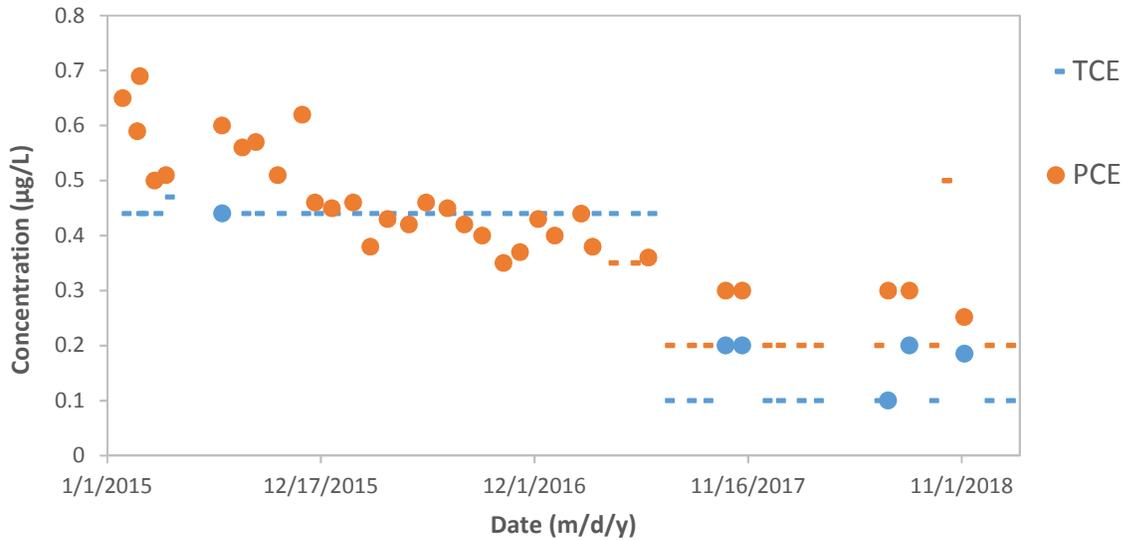
**Figure 2-5 TCE and PCE Concentrations in Well 11 Raw Water from January 2015 to January 2018 (dashed lines represent MDLs; dots represent reported concentrations)**
