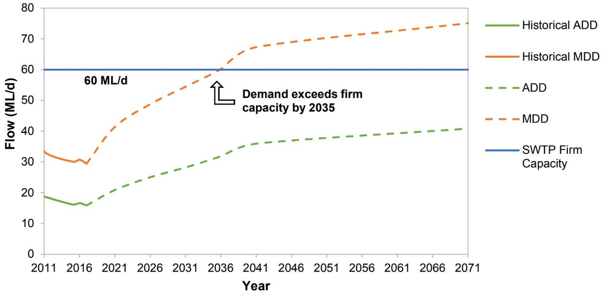
**Figure 4-2 City of Barrie 2018 Surface Water Demand Projections (Southern Zones: 2S, and 3S) compared to SWTP Firm Production Capacity**
