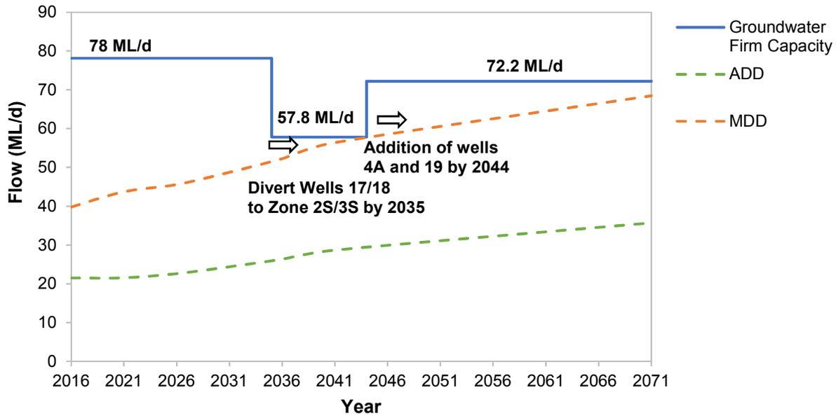
**Figure 5-5 City of Barrie 2018 Groundwater Demand Projections compared to Groundwater Firm Production Capacity (Northern Zones: 1, 2N, and 3N) with the implementation of Alternative 6A**
