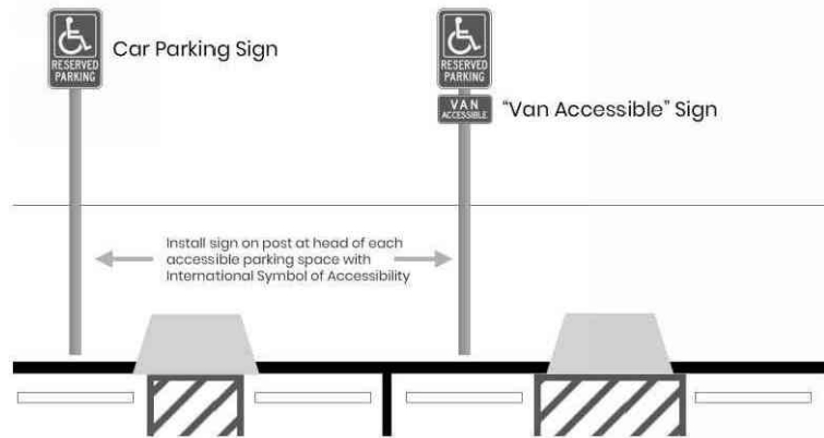
BARRIER FREE PARKING SIGNAGE SCALE: 1:30 5
