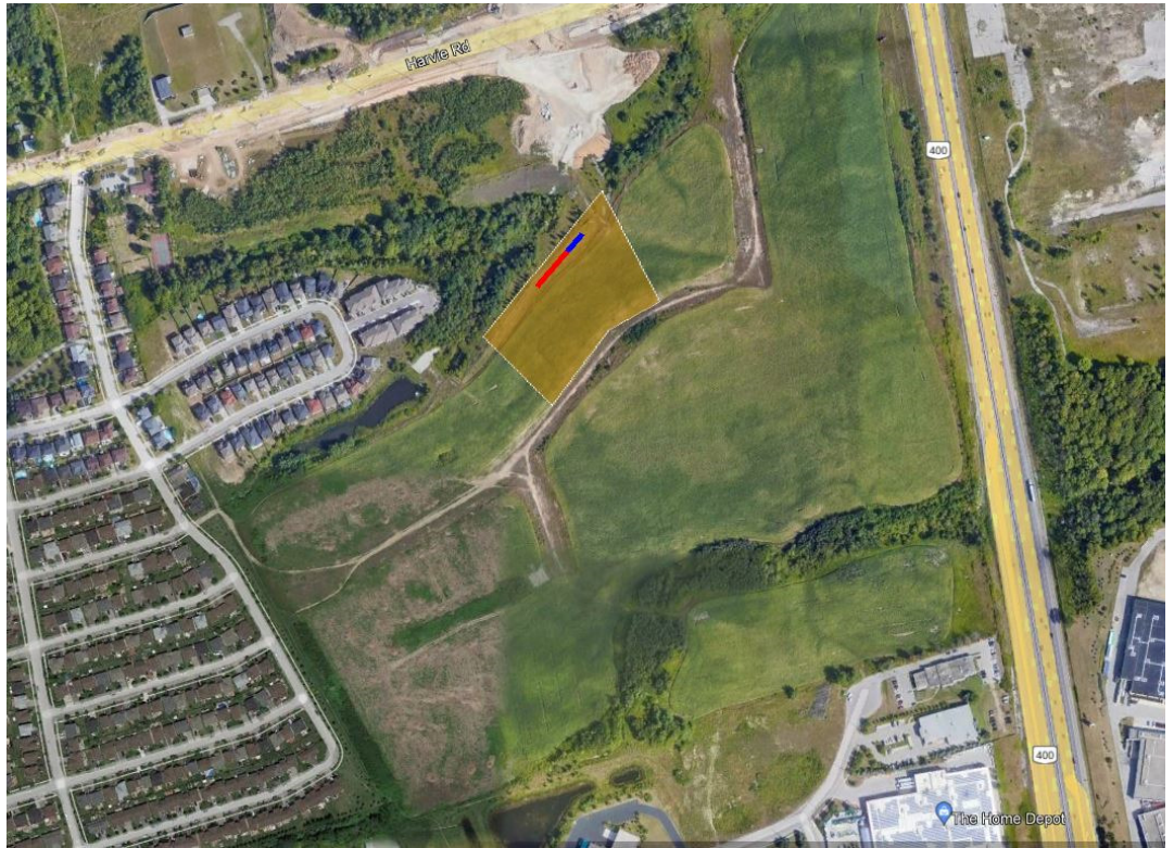
Figure 1: Survey area (yellow) with 1-meter MASW spacing marked (blue) and 3-meter spacing marked (red and blue)
