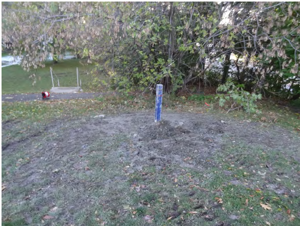
Photograph No. 8 – Monitoring well at Borehole BH2, West View
