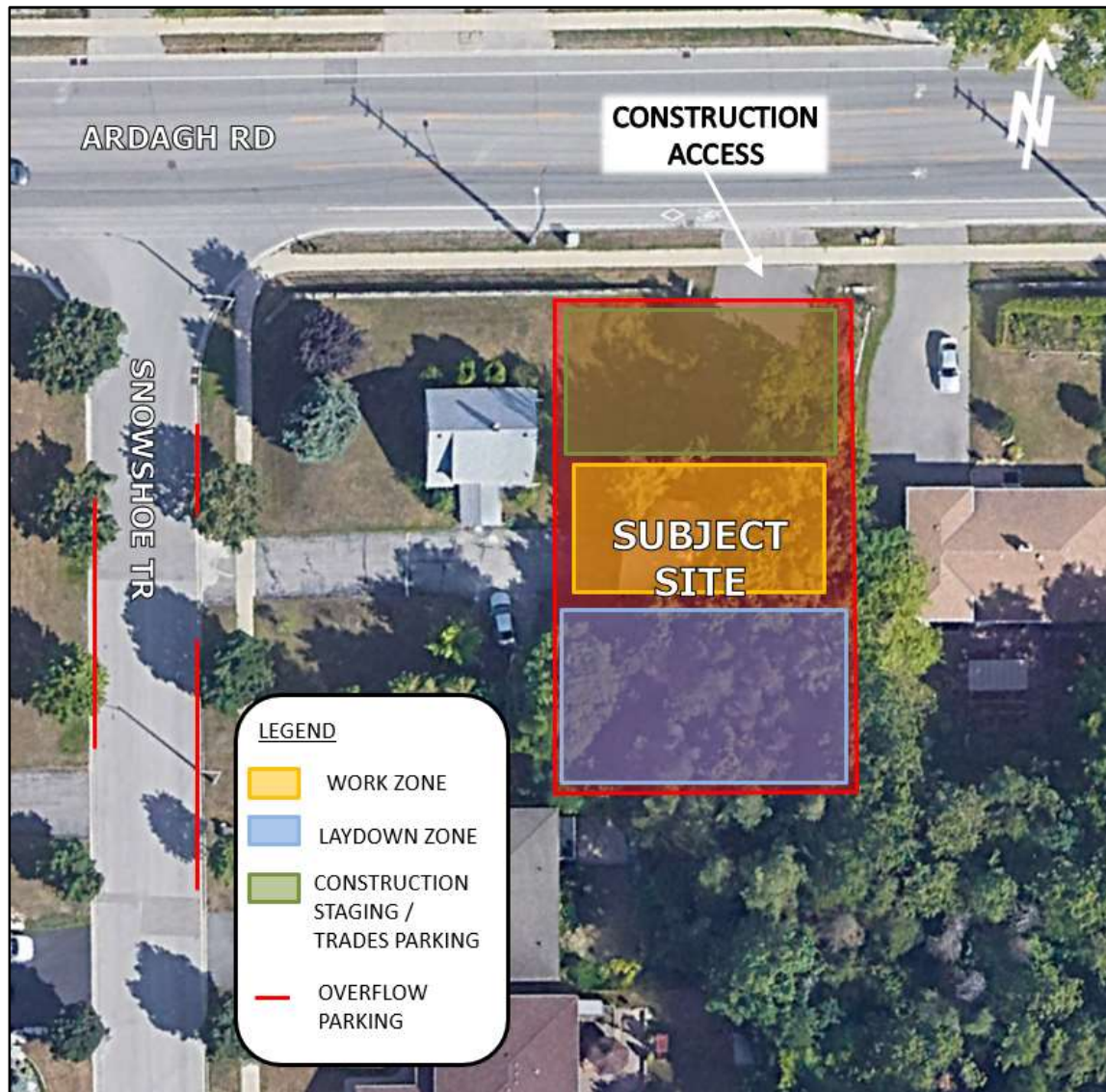
Figure 2 – Construction Staging Plan
