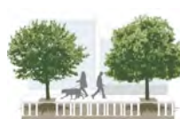
11 GREEN INFRASTRUCTURE UTILIZES UNDERGROUND SOIL CELLS FOR NEW TREE PLANTINGS AND TO CLEAN STORMWATER FROM THE ROADWAY.
