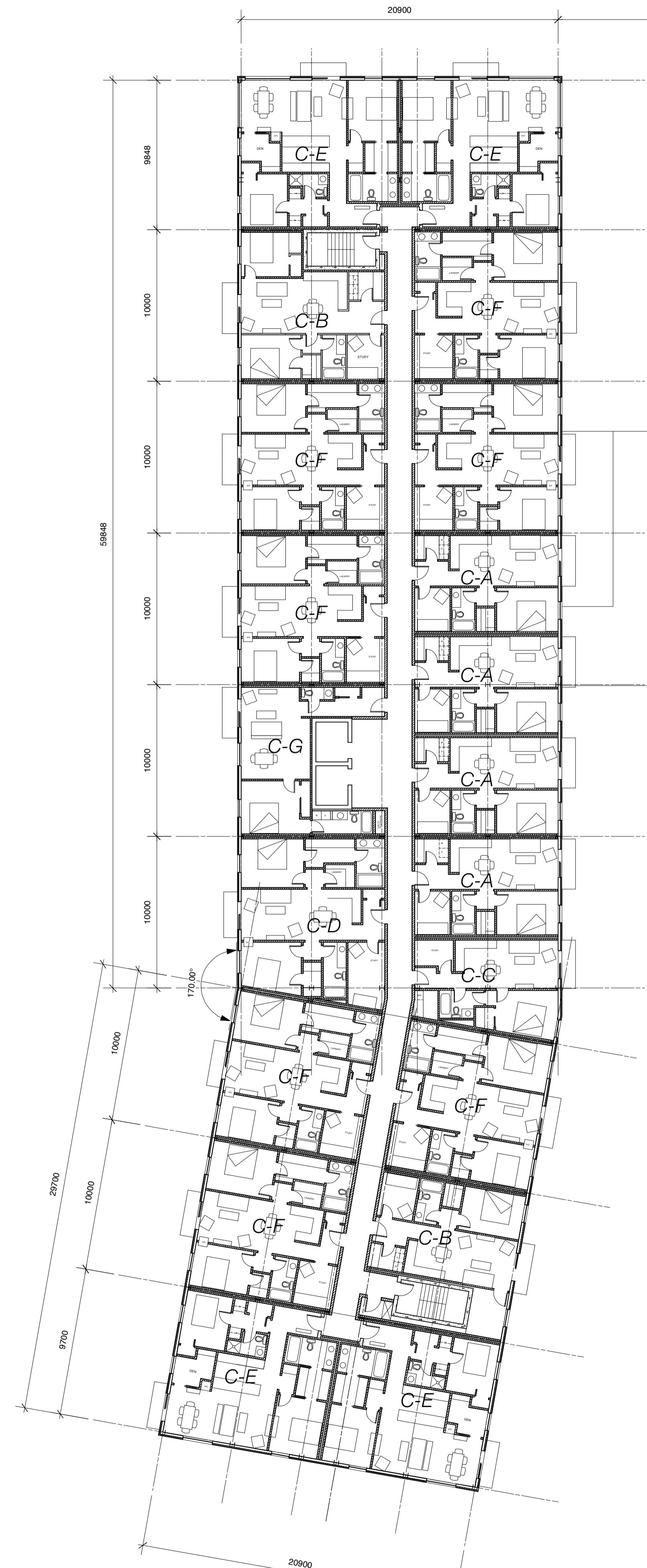
1 SENIORS CONDO TYPICAL FLOOR - 3-7 Scale: 1:200 GROSS FLOOR AREA: 1963 SQM/FLR; 9815 SQM TOTAL UNIT TYPE AREA # C-A, 1BR/DEN 66 SQM 20 C-B, 1 BR/DEN 84 SQM 10 C-C, 1BR/DEN 61 SQM 5 C-D, 2BR/DEN 107 SQM 5 C-E, 2BR/DEN 108 SQM 20 C-F, 2BR/DEN 89 SQM 35 C-G, 1BR 70 SQM 5 TOTAL 3RD-7TH FLRS 100 units
