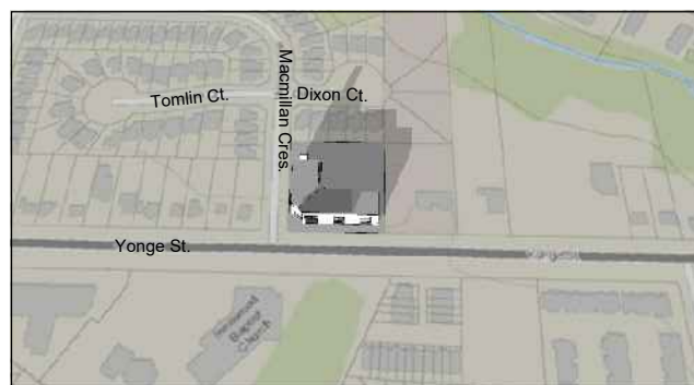
6:00pm, March 8 Shadow encroaching northeast onto residential properties along Dixon Ct. and Yonge St.
