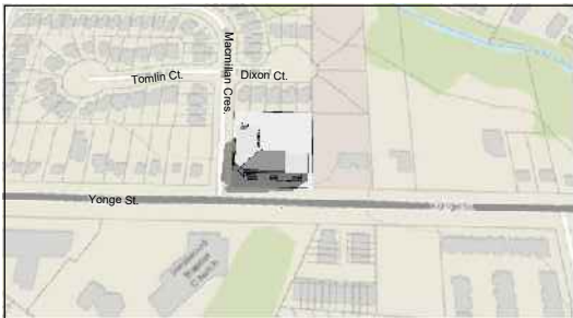
10:00am, June 21 Shadow encroaching west onto Macmillan Cres., and Yonge St., no impact on surrounding properties.
