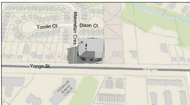
10:00am, September 21 Shadow encroaching west onto Macmillian Cres., no impact on surrounding properties.
