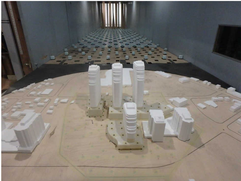
PHOTOGRAPH 2: STUDY MODEL INSIDE THE GWE WIND TUNNEL LOOKING UPWIND
