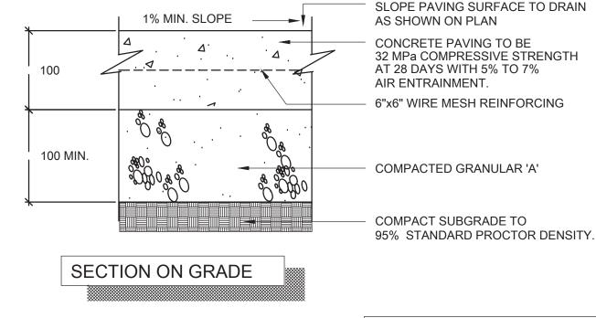
PROVIDE CLEAN STRAIGHT EXPANSION JOINT BETWEEN EXISTING AND NEW CONCRETE PAVING OR EXISTING STRUCTURE. EXPANSION JOINTS AT 6.0M MAXIMUM INT. CONTRACTION JOINTS AT 3.0M MAX. INT.
