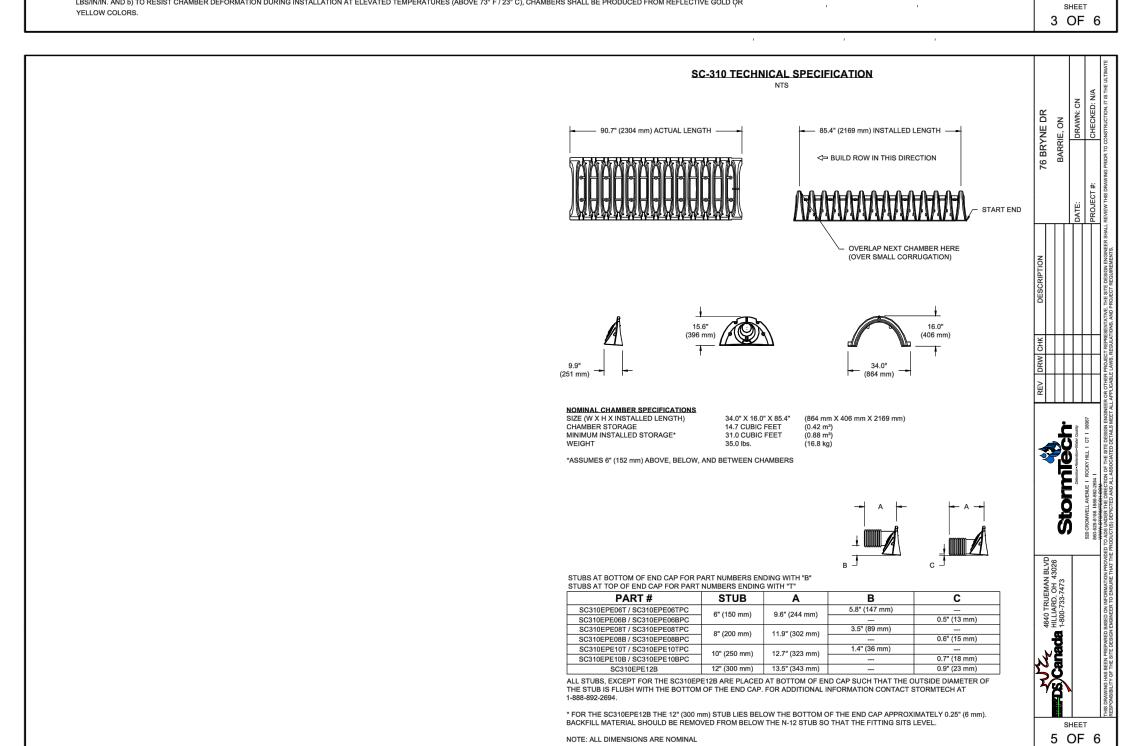
TO ENSURE THE INTEGRITY OF THE ARCH SHAPE DURING INSTALLATION, a) THE ARCH STIFFNESS CONSTANT AS DEFINED IN SECTION 6.2.8 OF ASTM F2922 SHALL BE GREATER THAN OR EQUAL TO 400 LBS/IN/IN, AND b) TO RESIST CHAMBER DEFORMATION DURING INSTALLATION AT ELEVATED TEMPERATURES (ABOVE 73° F / 23° C), CHAMBERS SHALL BE PRODUCED FROM REFLECTIVE GOLD OR
