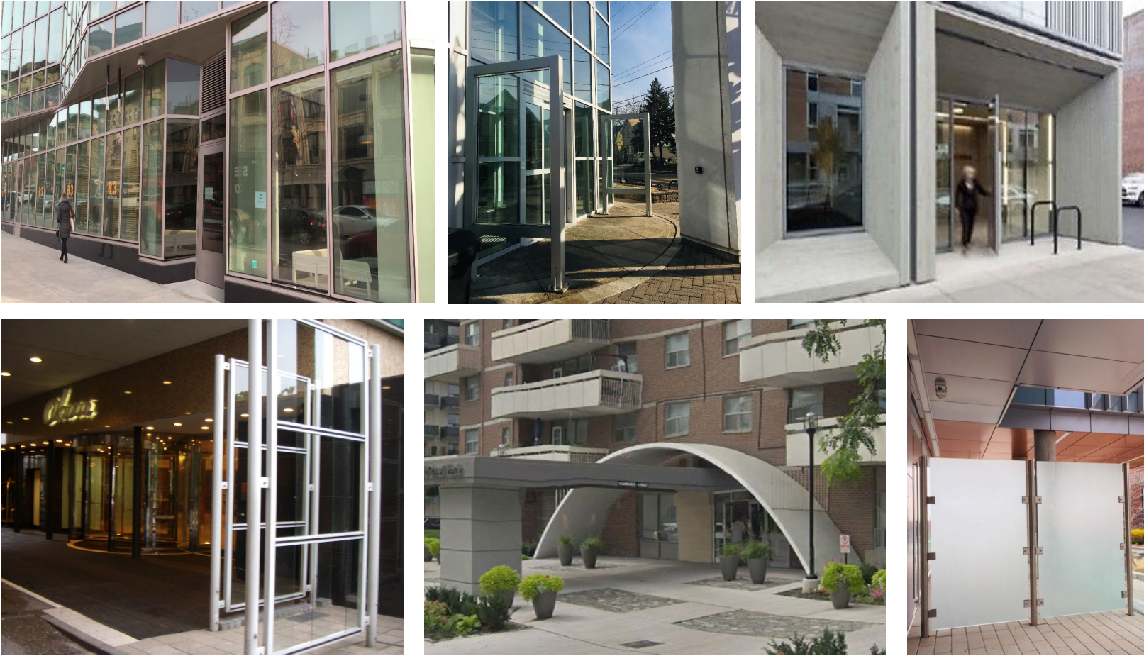
Image 10: Suggestions for wind control at the entrance for building A1
