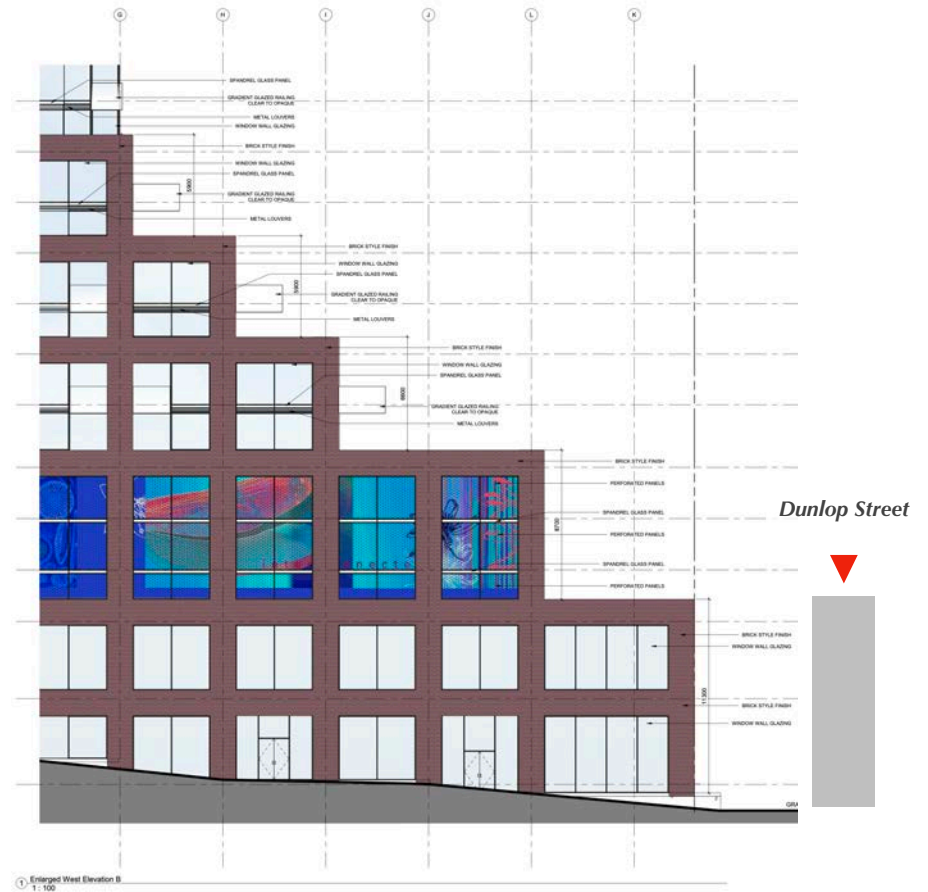
West elevation (portion): Showing a portion of the sloping site condition along Owen Street. The gradual transition in height from the tower level provides a more appropriate relationship with the subject heritage property to the south. The 4.5m height established here is in line with the Dunlop Historic Streetscape
