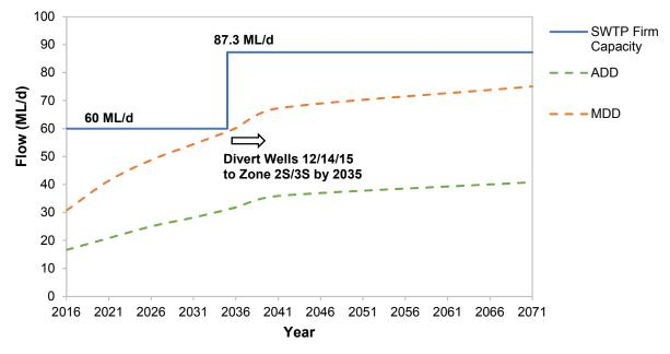
Figure 5-8 City of Barrie 2018 Surface Water Demand Projections Compared to SWTP Firm Production Capacity (Southern Zones: 2s, and 3S) with the implementation of Alternative 6B
