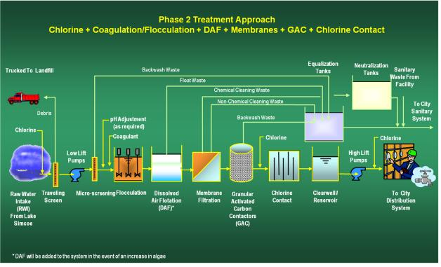
**Figure 2-3 Process Schematic of Surface Water Treatment Plant** A summary of the SWTP treatment train is presented in Table 2-3.
