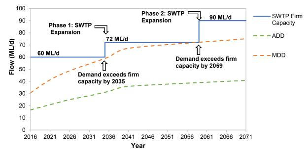
Figure 5-1 City of Barrie 2018 Surface Water Demand Projections compared to SWTP Firm Production Capacity (Southern Zones: 2S, and 3S) with the implementation of Alternative 4
