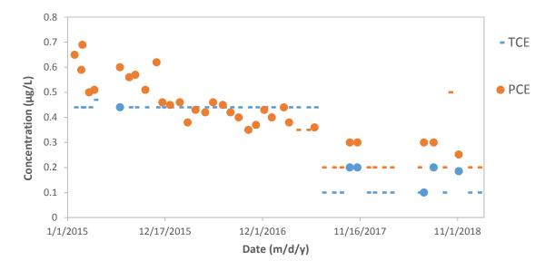
Figure 2-5 TCE and PCE Concentrations in Well 11 Raw Water from January 2015 to January 2018 (dashed lines represent MDLs; dots represent reported concentrations)
