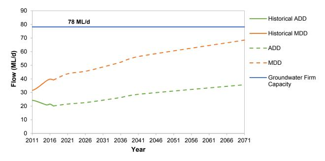
Figure 4-1 City of Barrie 2018 Groundwater Demand Projections (Northern Zones: 1, 2N, and 3N) compared to Groundwater Firm Production Capacity
