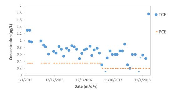
Figure 2-7 TCE and PCE Concentrations in Well 14 Raw Water from January 2015 to January 2018 (dashed lines represent MDLs; dots represent reported concentrations)
