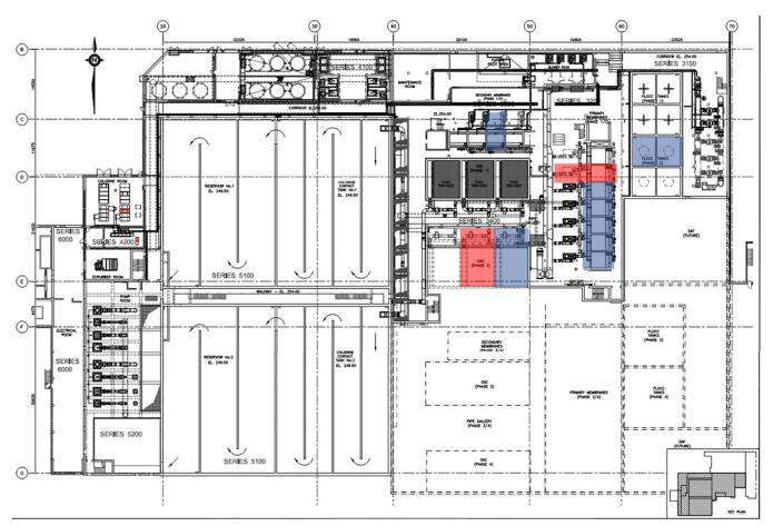
Figure 5-10 SWTP Plan View With Required Upgrades Highlighted in Blue for the Phase 1 Expansion, and in Red for the Phase 2 Expansion
