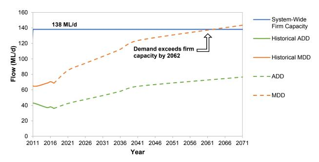
Figure 4-3 City of Barrie 2018 System-Wide Water Demand Projections compared to System-Wide Firm Production Capacity
