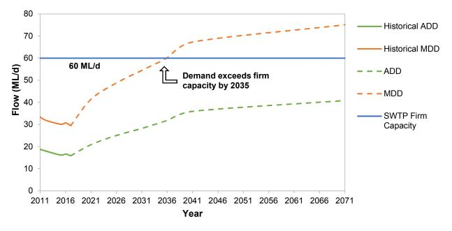
Figure 4-2 City of Barrie 2018 Surface Water Demand Projections (Southern Zones: 2S, and 3S) compared to SWTP Firm Production Capacity
