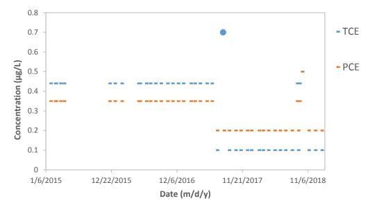
Figure 2-6 TCE and PCE Concentrations in Well 12 Raw Water from January 2015 to January 2018 (dashed lines represent MDLs; dots represent reported concentrations)
