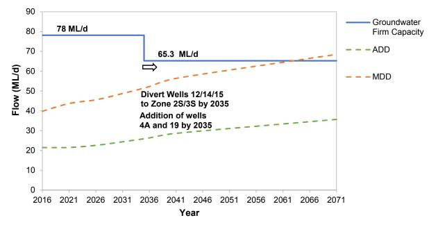
Figure 5-7 City of Barrie 2018 Groundwater Demand Projections Compared to Groundwater Firm Production Capacity (Northern Zones: 1, 2N, and 3N) with the implementation of Alternative 6B
