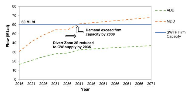
Figure 5-4 City of Barrie 2018 Surface Water Demand Projections compared to SWTP Firm Production Capacity (Southern Zones: 2S, and 3S) with the implementation of Alternative 5
