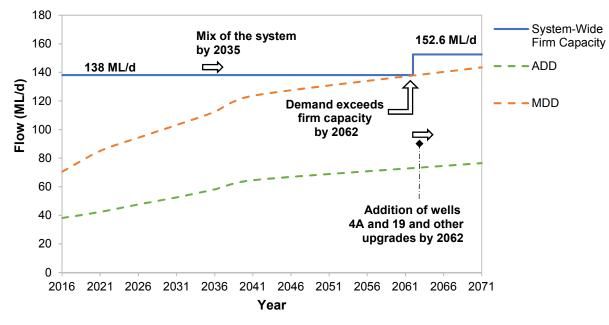
Figure 5-9 City of Barrie 2018 System-Wide Water Demand Projections compared to System-Wide Firm Production Capacity with the implementation of Alternative 7
