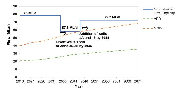
Figure 5-5 City of Barrie 2018 Groundwater Demand Projections compared to Groundwater Firm Production Capacity (Northern Zones: 1, 2N, and 3N) with the implementation of Alternative 6A
