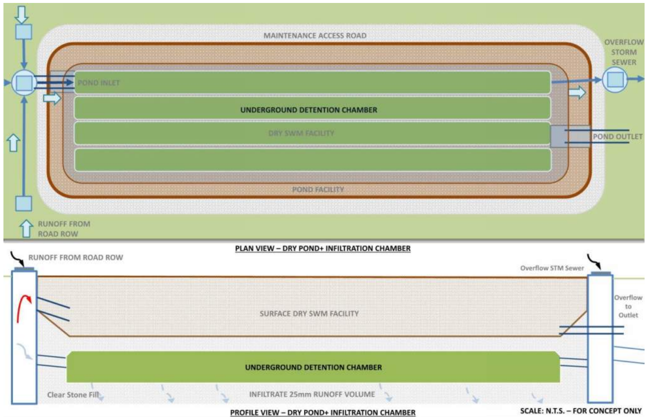
Exhibit 6-1 Infiltration Chamber Under Dry Pond
